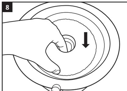
Place filter on top of filter holder, and press down firmly.
