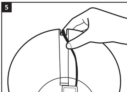
Re-thread power cord into groove in base.
