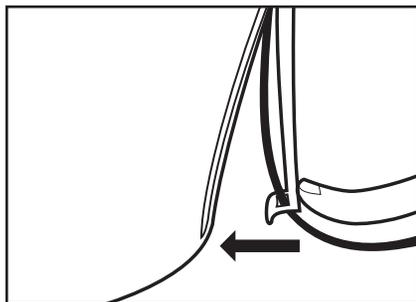
Slide power cord holder into groove in base. Ensure notches on the outside tip of the power cord holder line up with notches on outside of base, then press down firmly to lock into position.
